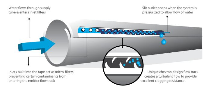
Most water will still contain foreign and organic particles even after it has been filtered. Therefore the design of the emitter is critical to help prevent clogging by stopping contaminants from entering the emitter.
