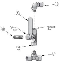
A. 1/4" 3-Way Ball Valve B. 1/4" x 1 1/2" Pipe Nipple C. 1/4" Pipe x 3/8" Tube Tee D. 1/4" Pipe x 3/8" Tube Elbow
