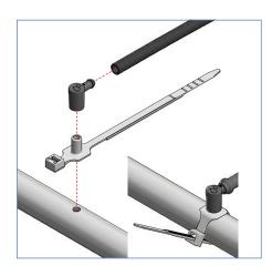
• PCJ with Press-Fit connector and elbow Press-Fit to barb adaptor
